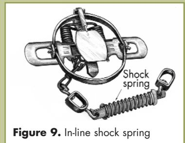
Figure 9. In-line shock spring
