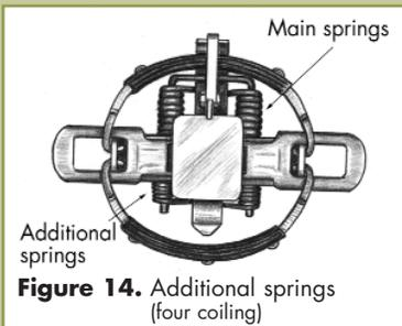
**Figure 14.** Additional springs (four coiling)
