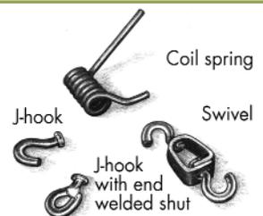
Figure 16. Trap components
