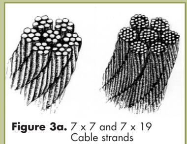
Figure 3a. 7 x 7 and 7 x 19 Cable strands
